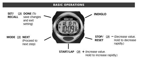
When setting, each button has a different function as indicated above. Display indicates when button changes function.
